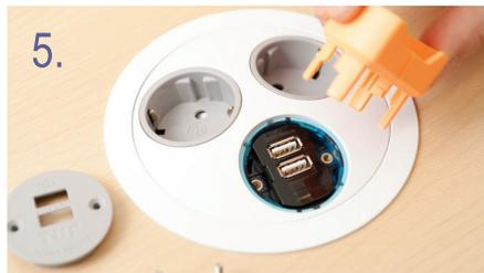
5. Insert the second part of the TUF Replacement tool until a click is heard (4 clips engage in TUF cartridge)
