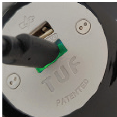
Green LED - Power Delivery 9V - 20V
