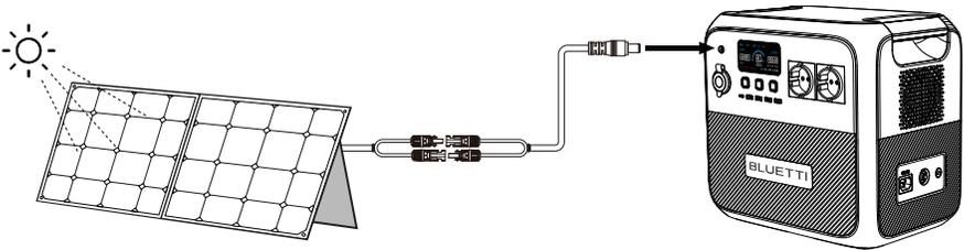
**Warning:** The open circuit voltage of solar panels cannot exceed 60V, otherwise it will damage the device(Note:It's not covered in the warranty)
